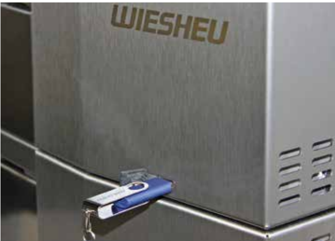
Programming of control unit via USB
